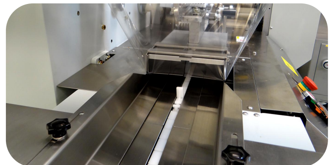
Delicate product conveyor with carrier card in-feed guide rails to handle product transitioning to the custom fixed former.
