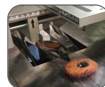
The Flow Wrapper 350T rapidly encloses the product in a tube of film before cutting and sealing the packages
